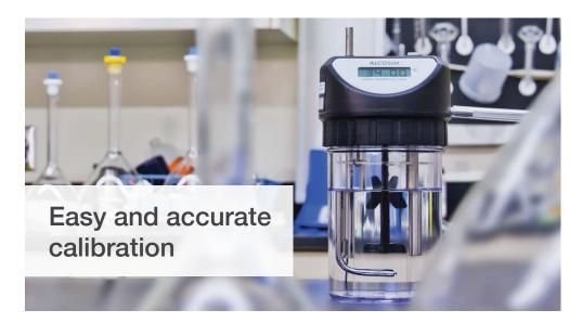
ALCOSIM is the easy and accurate way to calibrate or check-calibrate breath alcohol testing instruments. Carefully maintaining an alcohol reference solution, ALCOSIM produces an air-alcohol sample of precise concentration.
